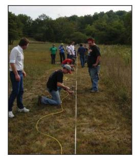
Figure 2. Wittenberg University geology students use Electrical Resistivity Ground Imaging to look for cave passages near the park.
