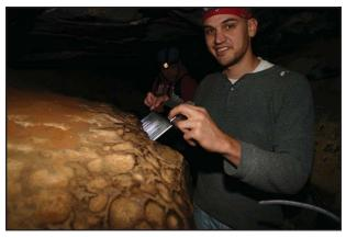
Figure 5. An Ohio State University geology student measures scallops to determine the speed and direction of the ancient cave rivers.
