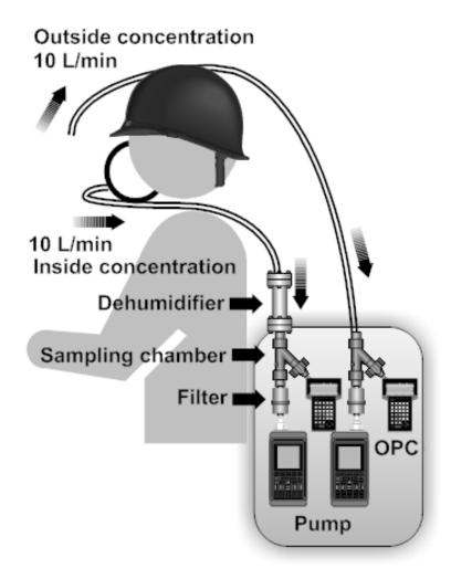
Figure 1. Schematic presentation of the personal sampling setup.
