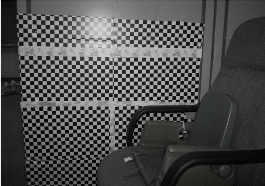
Figure 9. The set-up. Illustrated in this picture is the infant booster seat that participants were seated in during testing. The checkerboard pattern was used to measure arm movement.
