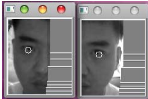
Figure 7. Demo of face extraction and finding eye using OpenCV
