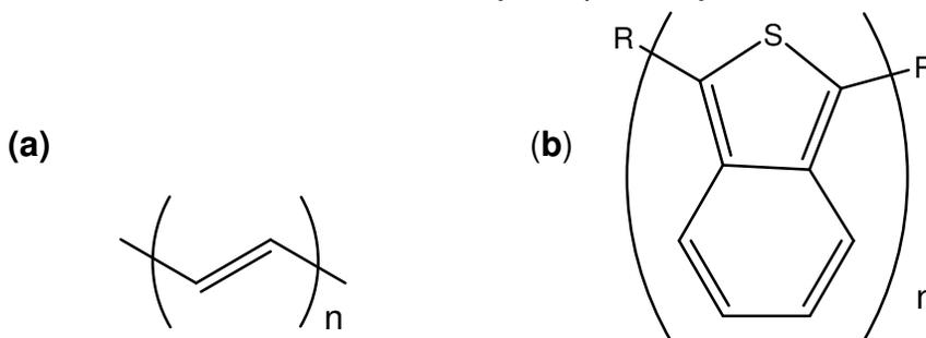
**Figure 1.8 (a) Polyacetylene; (b) Isothianaphthene**
