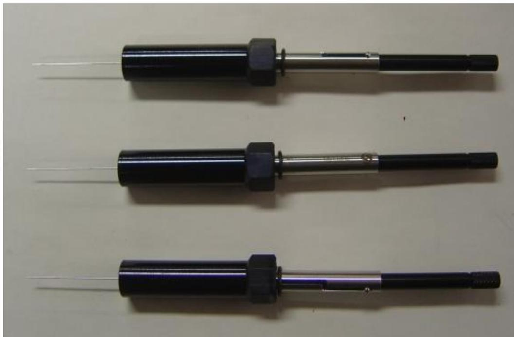
Figure 2.3. Supelco SPME needle with PA 85µm fiber.
