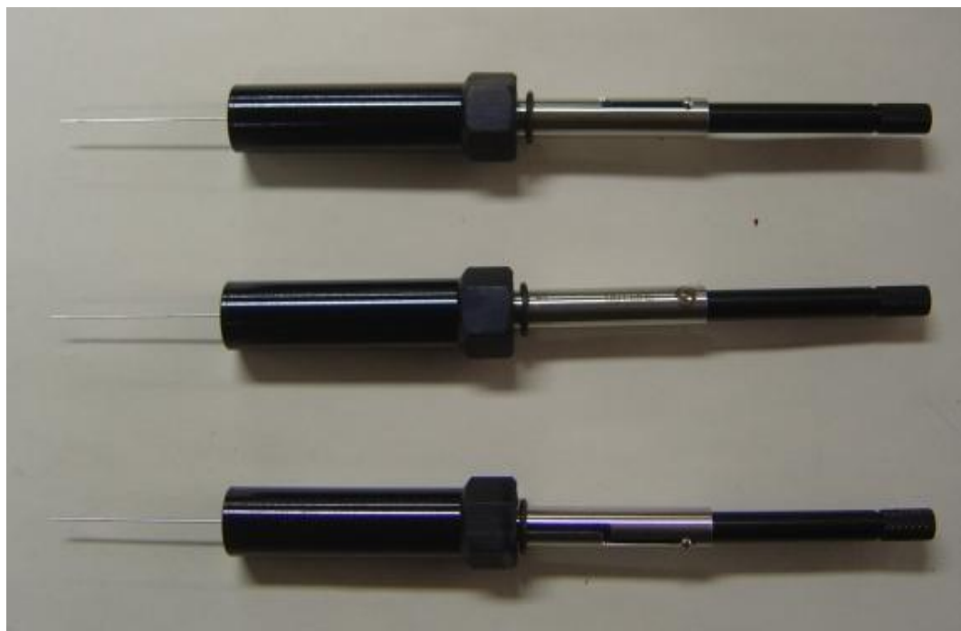
Figure 2.3. Supelco SPME needle with PA 85 \mu m fiber.
