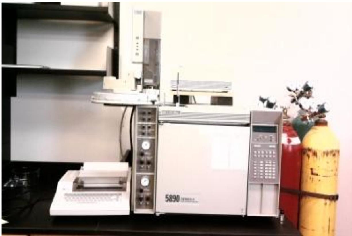
Figure 2.7. Analysis of chlorophenols by GC connected to HP 3396 series III integrator.
