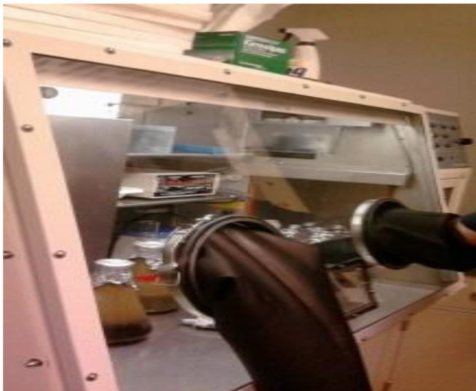
Figure 2.9. Forma Anaerobic system used for setting anaerobic conditions.
