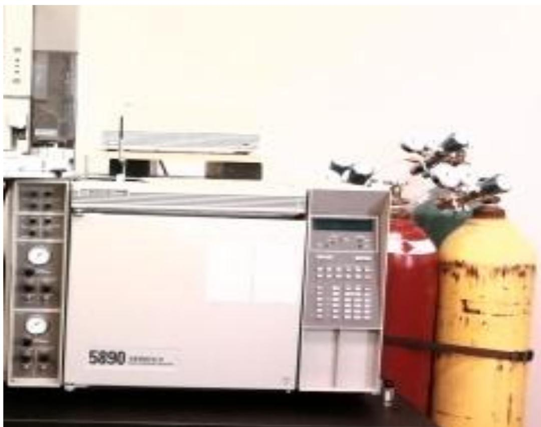
Figure 2.6. Gas Chromatograph-FID detector.
