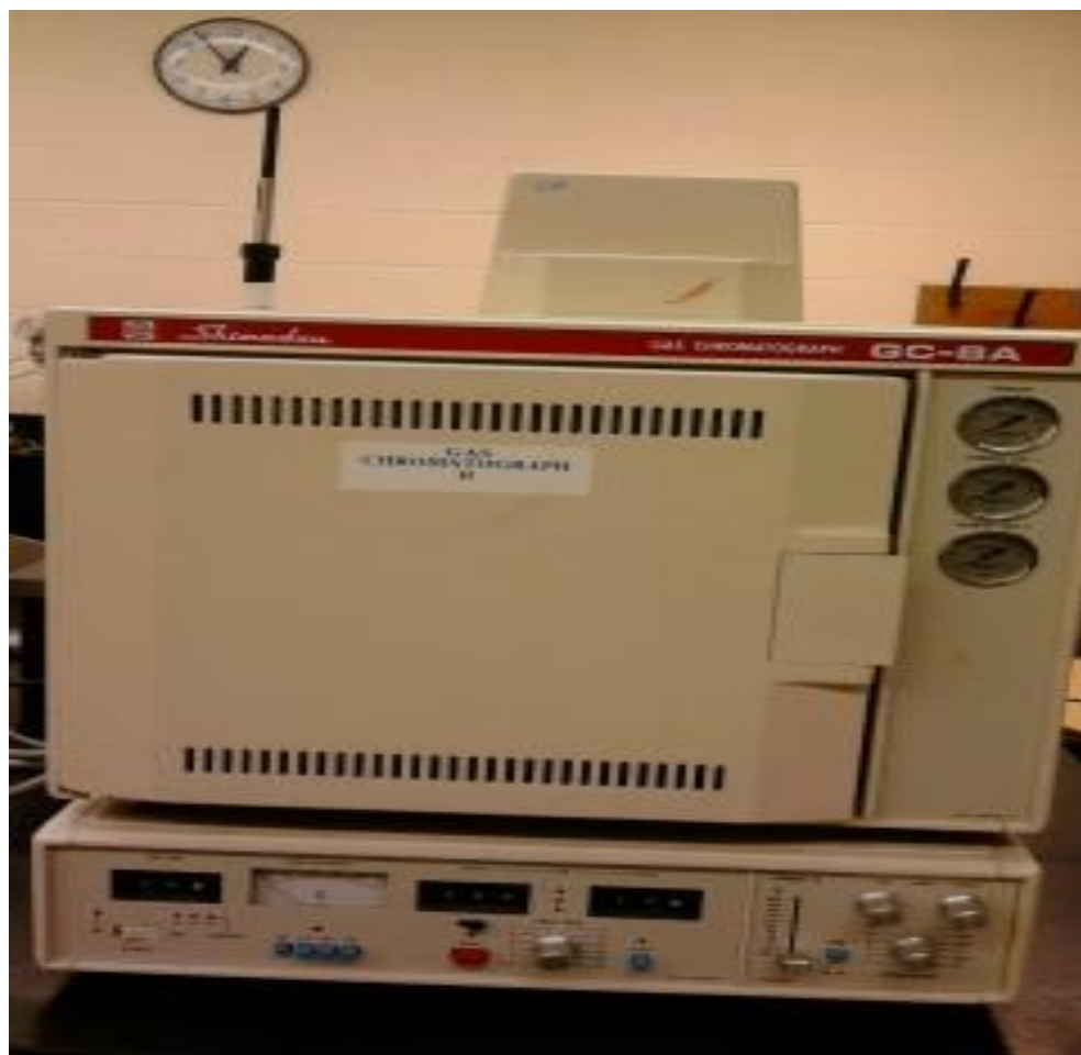
Figure 2.4. Fiber cleaning by using gas chromatograph.
