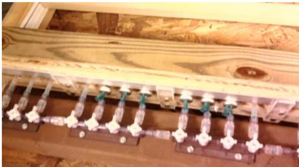
Figure 2.10. Nitrogen gas manifold.
