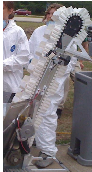
Figure 4b (Right): Conveyor as integrated into system
