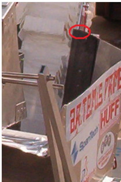
Figure 10: Rubber flap and foam insert conveyor-to-hopper sealing mechanism. (Red ellipse indicates location where foam is inserted.)
