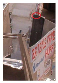
Figure 10: Rubber flap and foam insert conveyor-to-hopper sealing mechanism. (Red ellipse indicates location where foam is inserted.)
