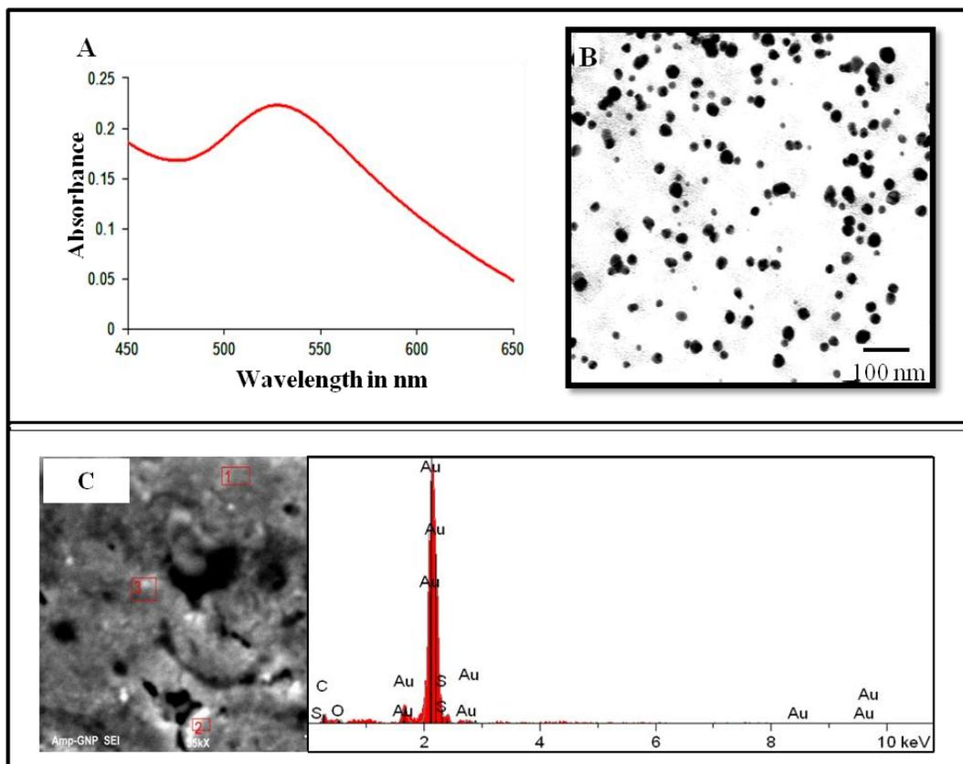
**Figure 1.** (A). UV-vis spectrum of Amp-GNPs with notable absorbance peak at ~540 nm. (B). Transmission electron microscope images of Amp-GNPs with average diameter of 15 nm. (C). Scanning electron microscope image and electron dispersion spectrum of Amp-GNPs. EDS shows the Amp-GNPs to be ~ 85% Au, ~ 8 % C, ~ 5 % O, and ~ 2 % S.
