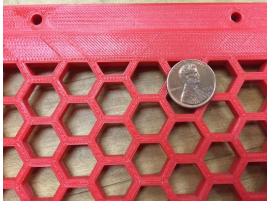
Figure 14 - 3-D printed pattern for head shell
