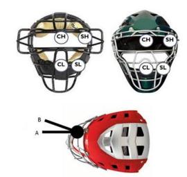
**Figure 3.** Ball/mask impact location and trajectory detail.
