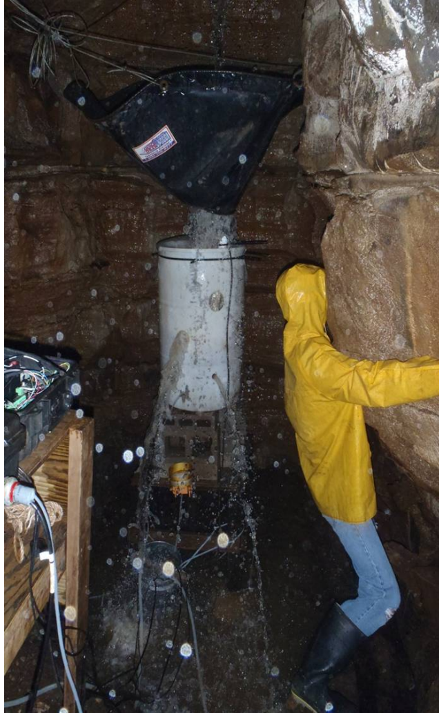
Figure 3.1 Discharge barrel and data logger set up at WF1 during spring storm event.
