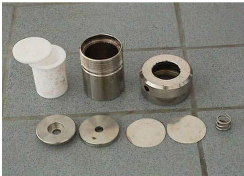
Figure 3. PTFE cup with cover, acid digestion bomb body, screw cap, pressure plate (upper), pressure plate (lower), corrosion and rupture discs, spring (from left to right).
