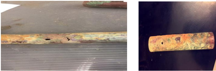
Figure 4: Corroded water pipe sample from Bowling Green, KY
