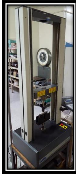
*Figure 3.* Chatillon DC 1000 compression/tensile tester
