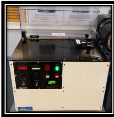
*Figure 9.* NOVA 1401 dielectric voltage breakdown tester
