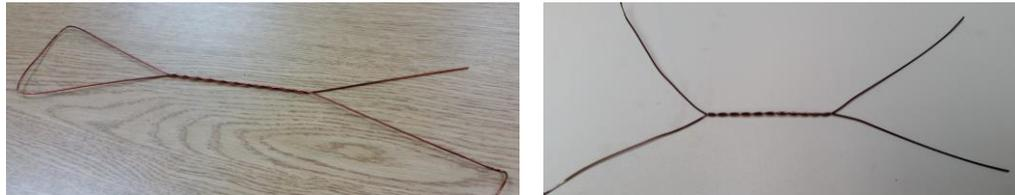
*Figure 8.* Cut the wire to create two independent circuits
