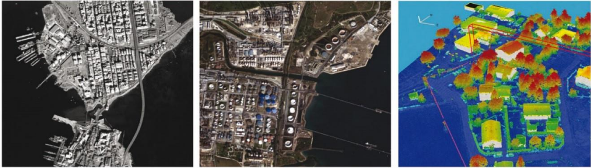
Figure 2.5. Differences in spectral resolution. The first image is from a panchromatic sensor. The middle image is from a multispectral sensor. The last image is from a LiDAR sensor. Source: McIntosh (2012).
