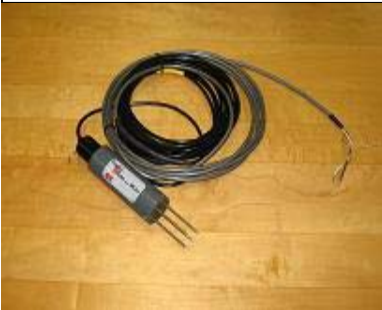
Figure 3: Probe for monitoring soil moisture levels.
