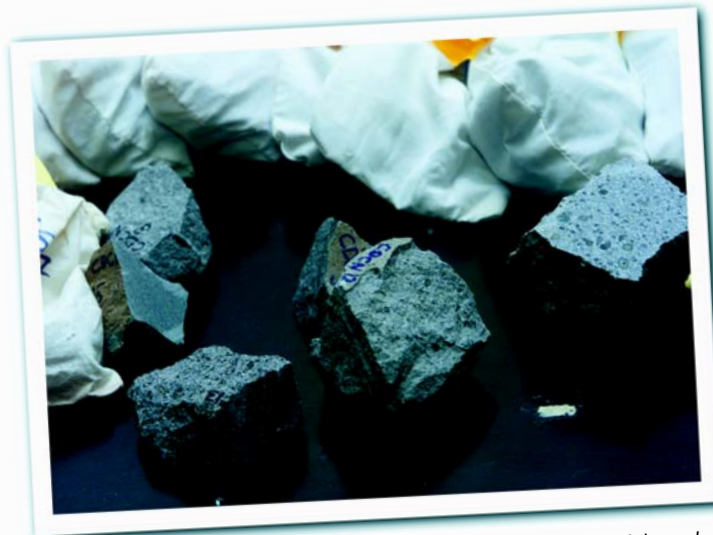
Samples of lava flows from a volcanic complex in Chile are cut into slabs and made into thin sections for microscope investigations. Portions of each sample are crushed, powdered, and melted for analysis of major and trace element composition, for isotope analysis, and age determinations.
