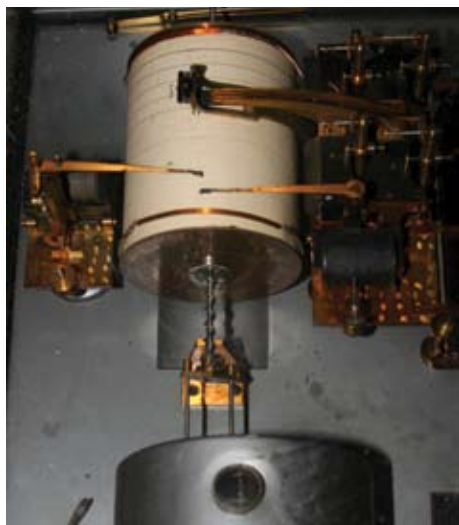
An antique Triple Register is used to measure sunshine, wind, and rainfall.
