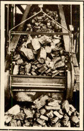
Boom over which prepared sizes are loaded into railroad cars after being screened for shipment.
