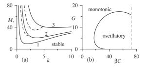
FIG. 1. (a) Marginal stability curves  $M_*(k)$  for G=10: solid lines correspond to the monotonic mode, dashed ones—to the oscillatory mode;  $\beta=1,10,40$  for lines 1, 2, and 3, respectively. (b) The domain of oscillatory instability. The dashed vertical line marks the boundary of the long-wave instability, Eq. (9).
