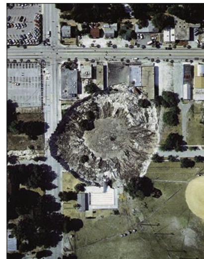
Figure 6.19: Sinkhole at Winter Park, Florida, near Orlando, which formed catastrophically in one day in 1981 (U.S. Geological Survey photo).
