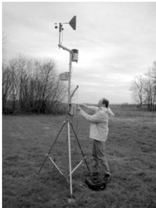
Figure 2. Weather station for recharge measurements, showing typical surface landscape above the cave system.
