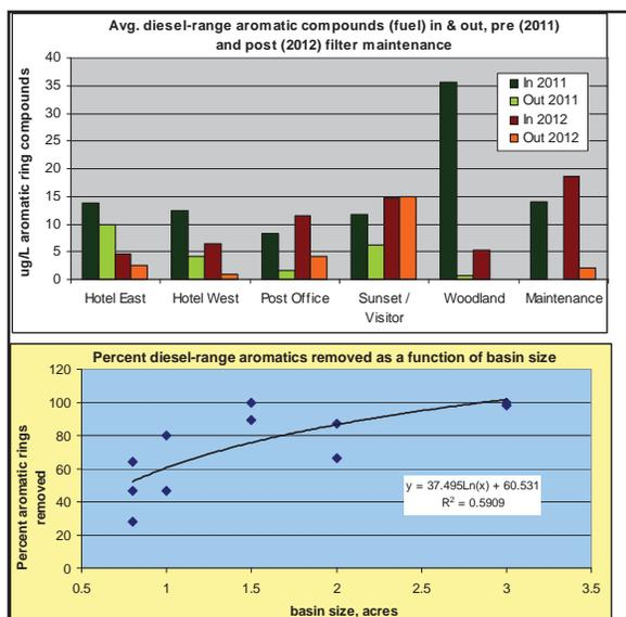
**Figure 1:** 1a(top graph): Average concentration of diesel range aromatic compounds dissolved in storm runoff at the filter inlets and outlets prior to and after the filters had been serviced in the late fall of 2011. [Sunset / Visitors is Sunset Lodge in 2011, and, Visitor Center in 2012; n = 3 or more] 1b (bottom graph): Regression analysis comparing the percent aromatic compounds removed by the filter as a function of parking lot size.
