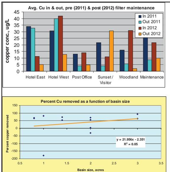
**Figure 3:** 3a (top graph): Average concentration of copper ( $\text{Cu}^{2+}$ ) dissolved in storm runoff at the filter inlets and outlets prior to and after the filters had been serviced in the late fall of 2011. [Sunset / Visitor bars are for Sunset Lodge in 2011, and, Visitors Center in 2012; n = 3 or more]. 3b (bottom graph): Regression analysis comparing the percent copper removed by the filter as a function of parking lot size.
