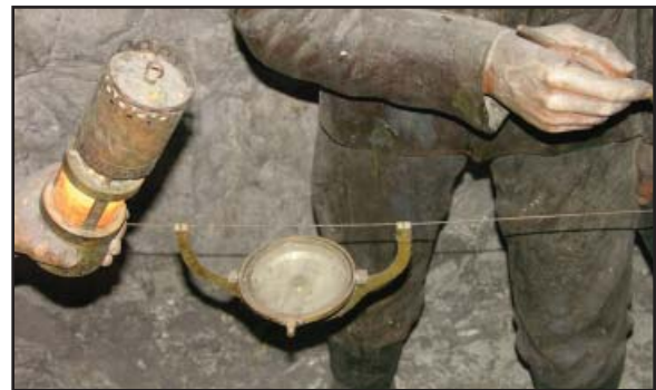
Figure 2: A mine survey display at the Deutsches Museum showing the use of a string mounted compass.
