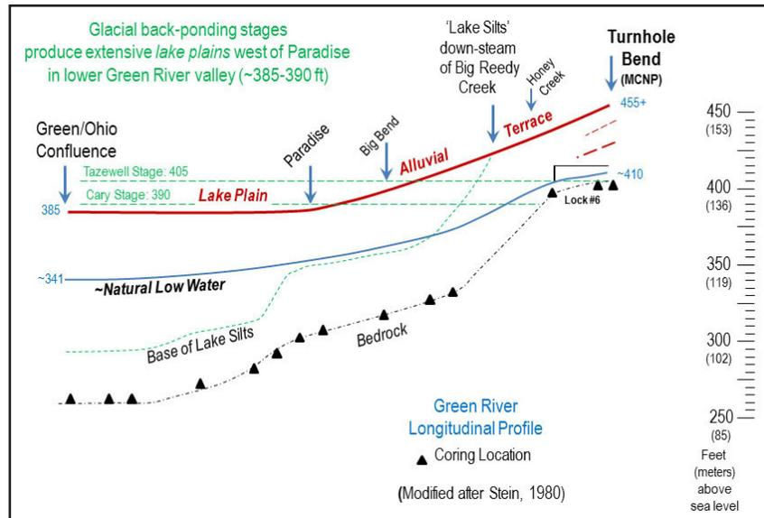
**Figure 2:** Green River longitudinal profile showing main alluvial terrace merging with lake plain formed by back-ponding during Tazewell and Cary glacial outwash stages on the Ohio River. The main alluvial terrace at Turnhole Bend lies 65-70 ft higher than the lake plain.
