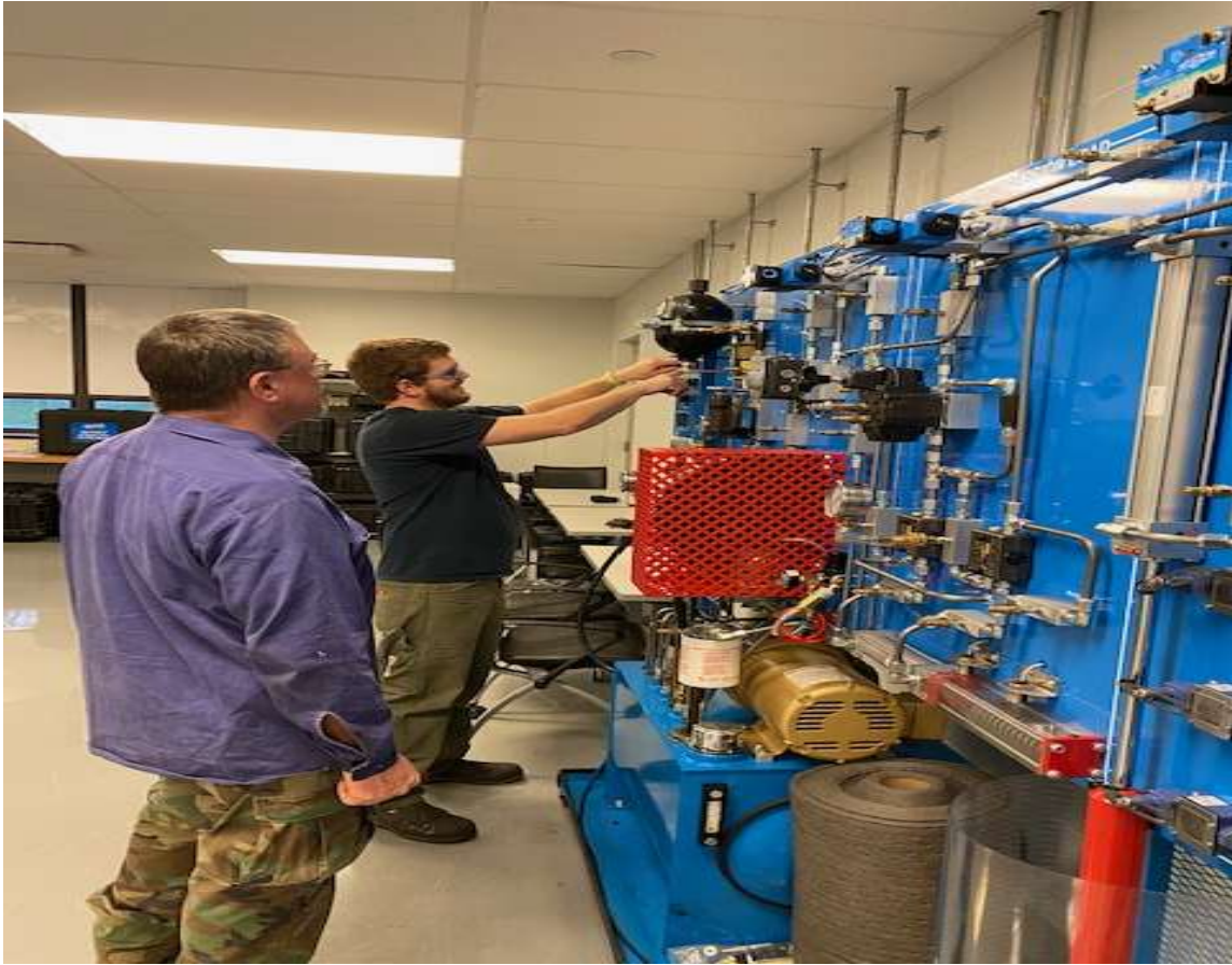
Figure 5. MAP and FAME students working with the hydraulic troubleshooting trainer.
