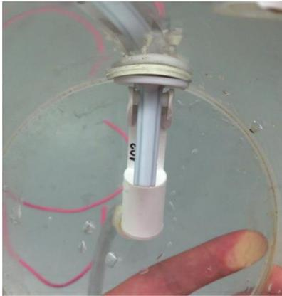
Figure 9: Float sensor installed with included installation parts
