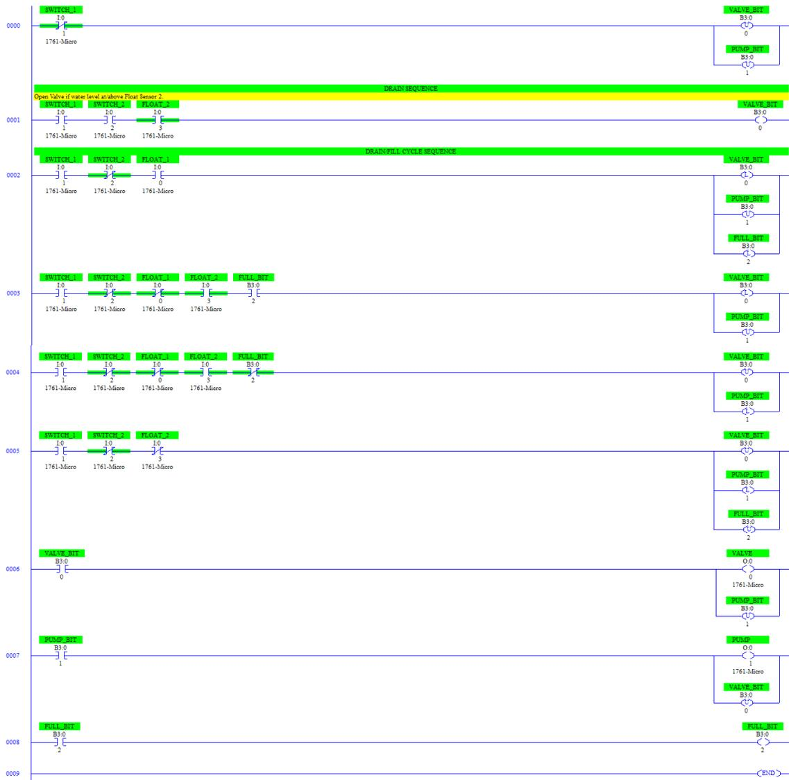
Figure 14: Complete Water Tank System Code
