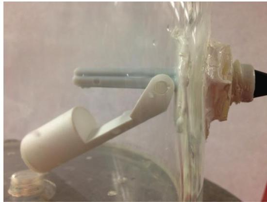
Figure 10: Float sensor installed with waterproof caulking
