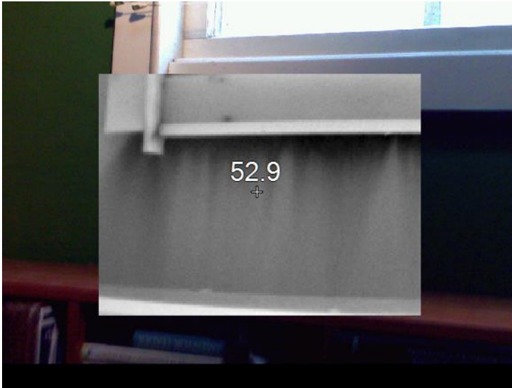
Figure A.2. Cold Air Infiltration around Coordinator Office Window. Source: Robert E. Choate. (2013). “Energy Audit Baseline Study”.
