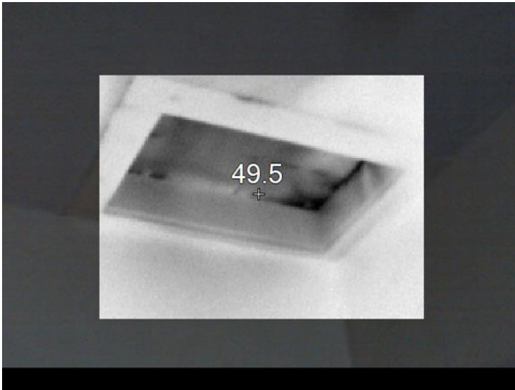
Figure A.5. Warm Air Escape through Attic Hatch. Source: Robert E. Choate. (2013). “Energy Audit Baseline Study”.
