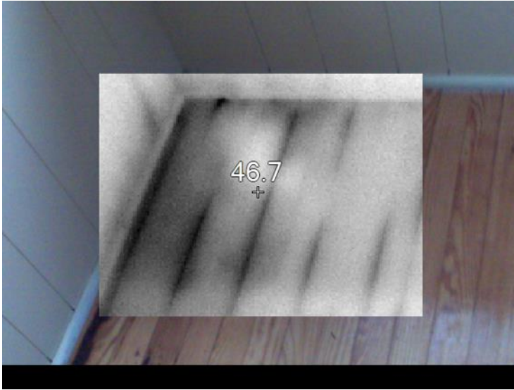
Figure A.10. Cold Air Infiltration around Sunroom Baseboards. Source: Robert E. Choate. (2013). "Energy Audit Baseline Study".
