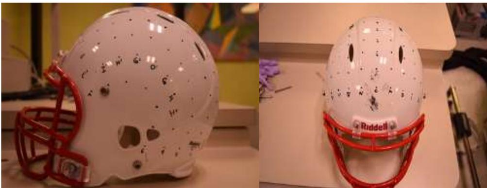
**Figure 1.** Image of helmets depicting transverse and longitudinal graphing of the accelerometers placement.
