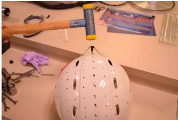
**Figure 4.** Small blunt flat tipped screw head and hammer used to create specific impact sight for testing.
