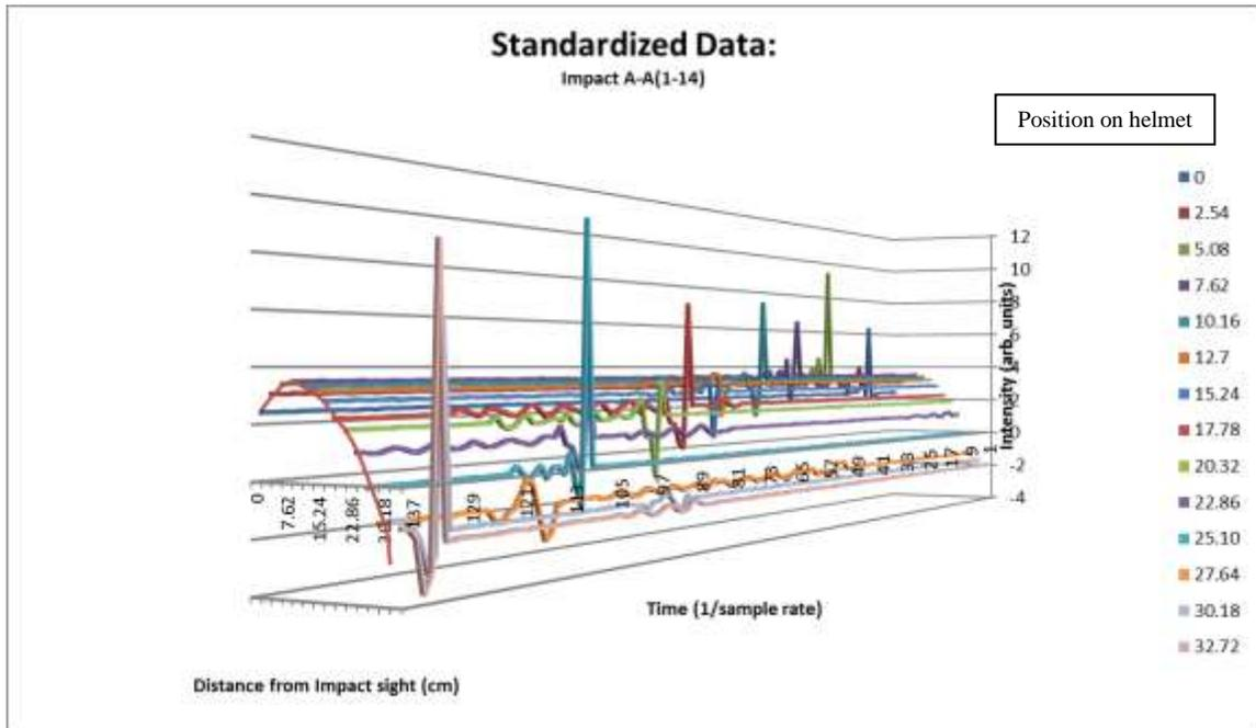
**Figure 9.** Standardized data of frontal impact propagation of plots along the A longitudinal line.
