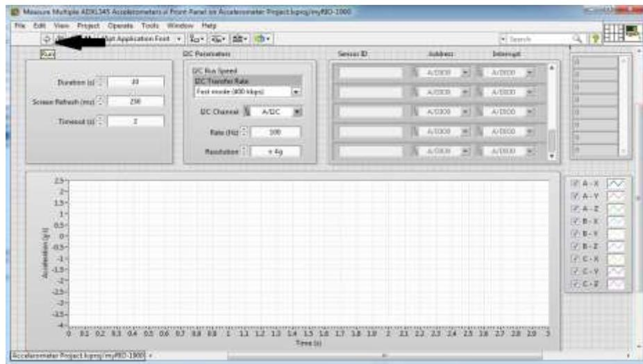
**Figure 3.** MyRio screen with arrow pointing to “Run”, which was used to record the data depicting 10 second duration with  $\pm 4g$  resolution
