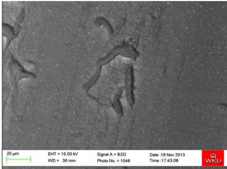
**Figure 8.** Observed damage of helmet surface after multiple impacts
