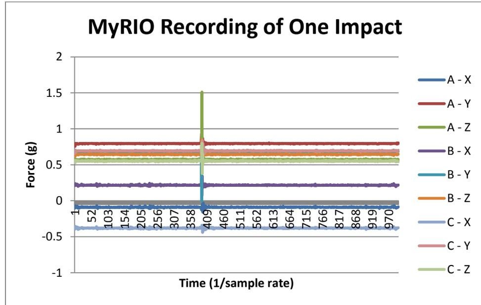
**Figure 5.** Single impact recording from the MyRIO. It recorded waves in the x, y, and z coordinates from accelerometers A,B, and C.
