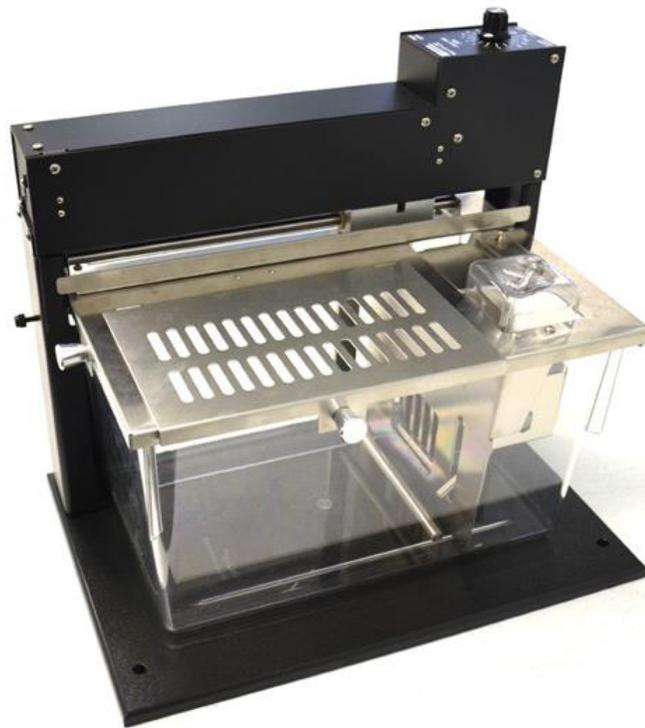
**Figure 2.** An automated sleep fragmentation chamber from Lafayette Instruments.
