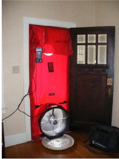
Figure 9. Blower Door Field Measurement Setup
