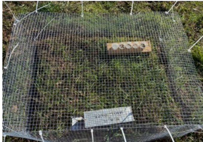
Figure 2.7 depicts the trial arena closed with the rodent trap from trial #1 set open and the seed cups present.
