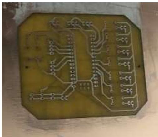
**Figure 25. Circuit Board in Production**
