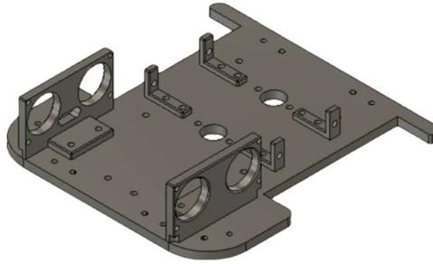
**Figure 2. Partial Skeleton of Autonomous Navigation Robot**
