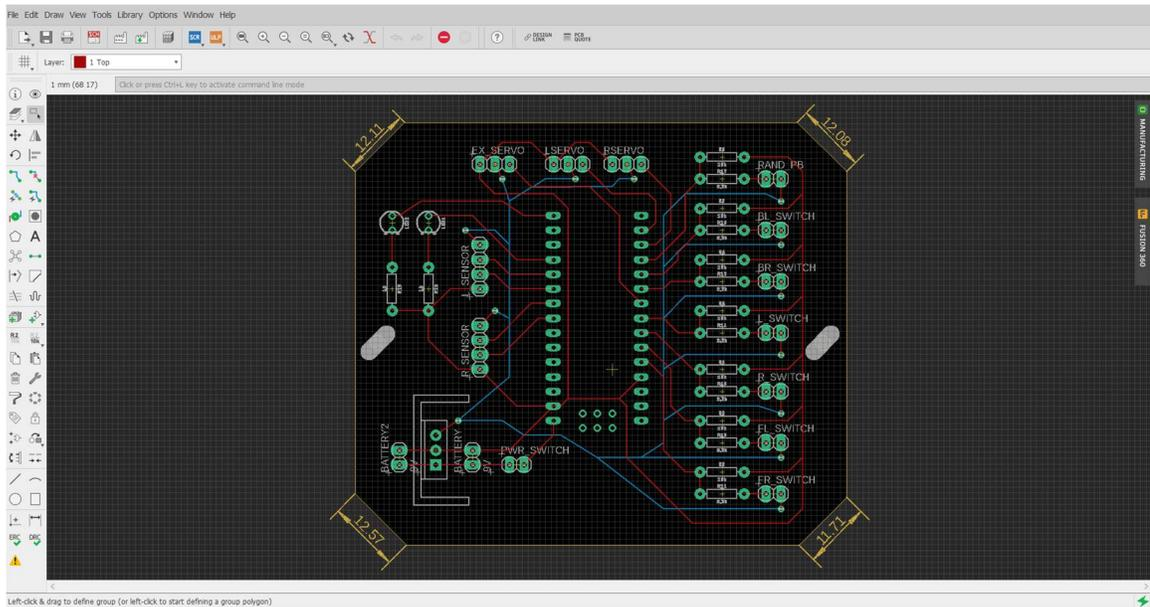
**Figure 23. Eagle Circuit Board Layout**
