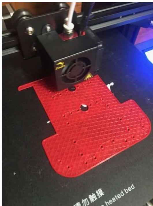
**Figure 24. 3-D Printer Producing Robot Base**
