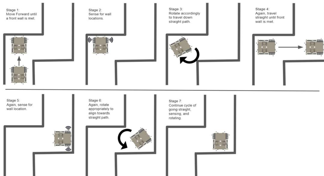
**Figure 11. Concept of Operation**
