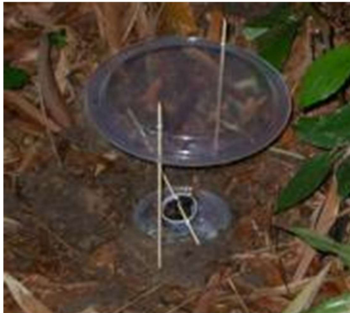
Figure 8. A conventional pitfall trap with a rain roof created using kebab sticks and a plastic plate.
