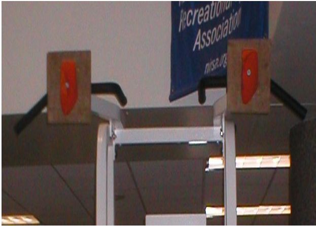
Figure 3a. (above) Anterior view of the climbing-specific training device prototype, attached to the WAPU machine. The prototype was made of wood, and displays two orange, pinch grip climbing holds.
