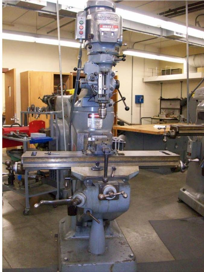
*Figure 2.* Milling machine
