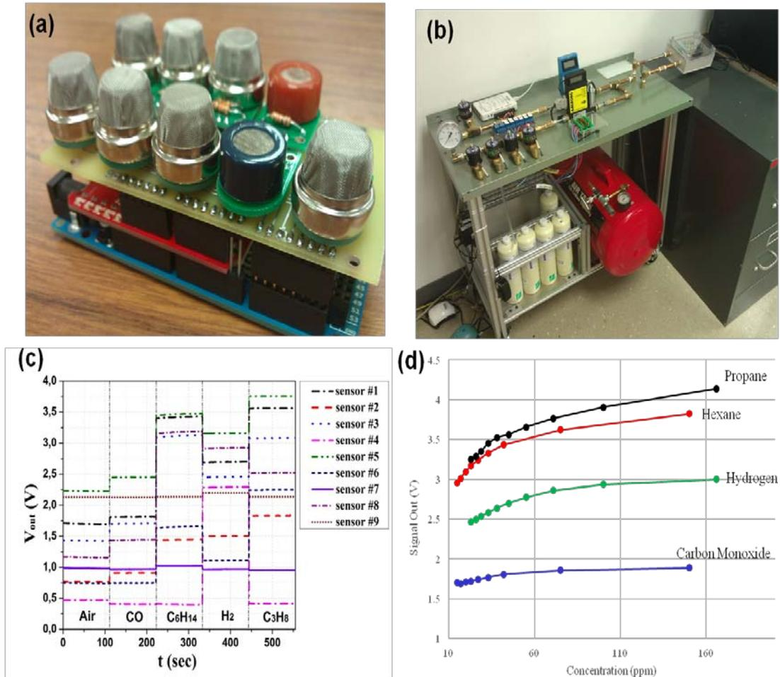
**Figure 3.** (a) Integrated multi-sensory systems based on  $\text{SnO}_2$  gas sensors developed at the Applied Physics Institute (b) calibration and testing system, (c) integrated response of a multi-sensory system, (d) MQ-2 sensor output signal upon exposure to different gases as a function of concentration.
