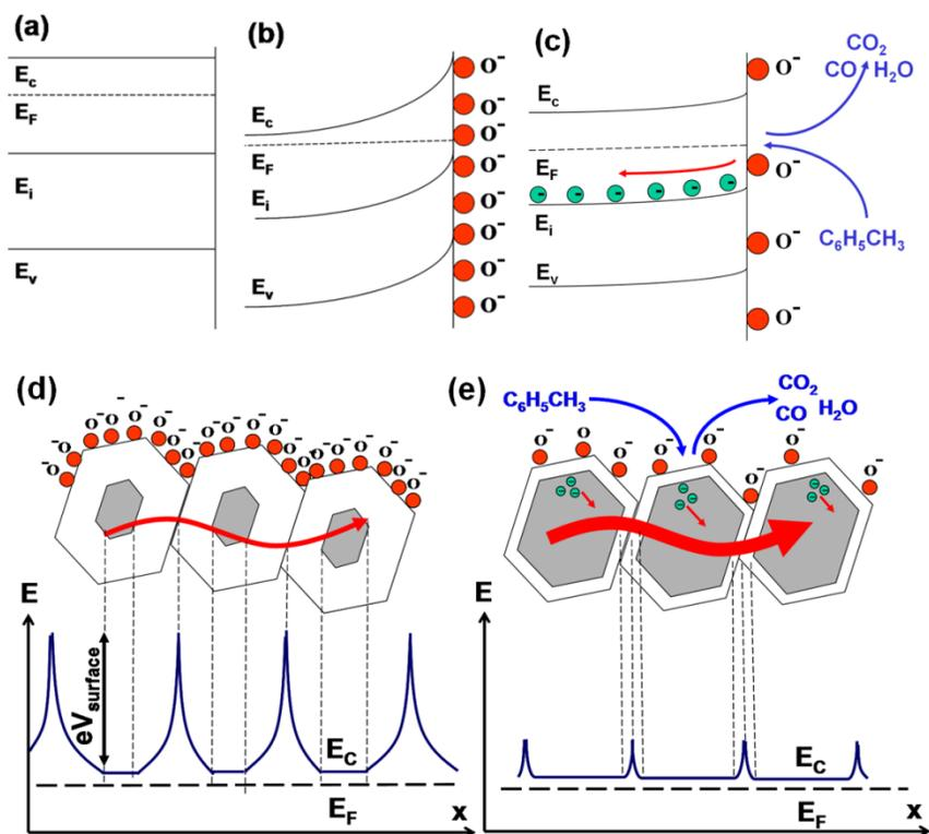
**Figure 2: Top:** Energy band diagrams of (a) bulk  $SnO_2$ , (b) at the surface of  $SnO_2$  with  $O^-$  termination and (c) upon exposure to toluene. **Bottom:** Schematic energy-level diagrams of the polycrystalline  $SnO_2$  layer (d) prior to exposure to toluene and (e) after exposure and subsequent oxidation of toluene.
