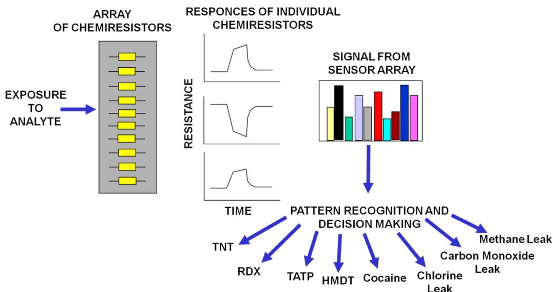
**Figure 1:** Principle of operation of an integrated chemical sensor (electronic nose).
