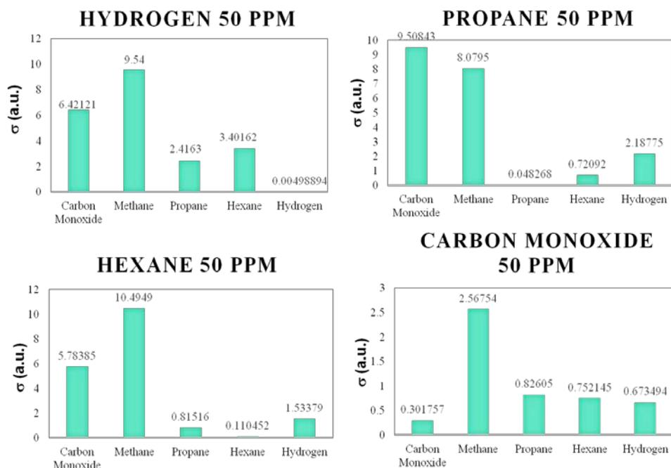
**Figure 4.** Standard deviation upon the exposure to various analytes. Minimum standard deviation corresponds to the detected analyte.
