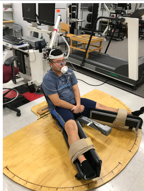
Figure 3. Participant performing the movement task using the stretching apparatus and metabolic cart.
