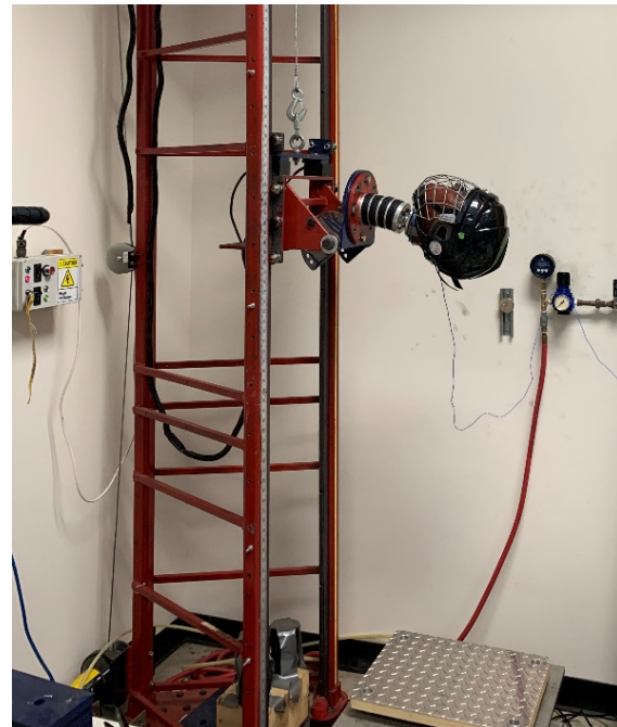
Figure 2. Setup of the head impact simulation testing.
