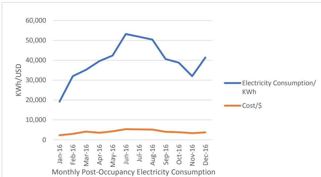
Figure 4. Post Occupancy Monthly Electricity Consumption and Cost for Augenstein Alumni Center
