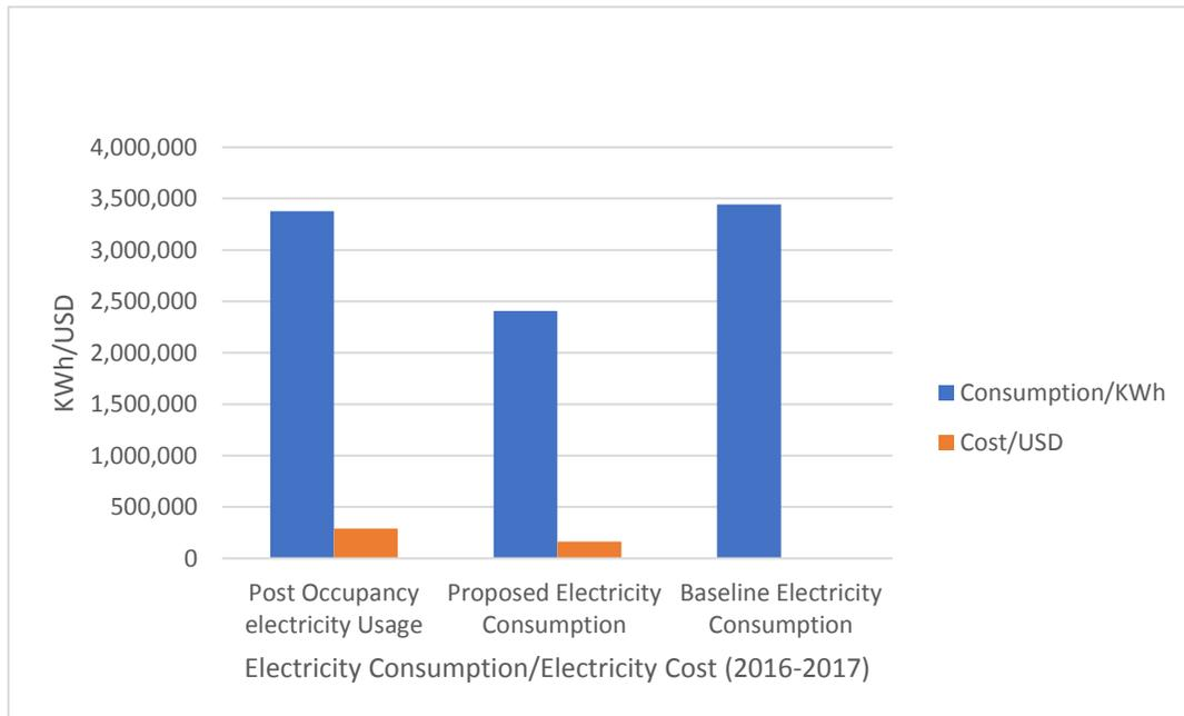
*Figure 1.* Comparison Between Post-Occupancy Electricity Usage and Pre-Construction LEED Model at DSU (April 2016 -April 2017)
