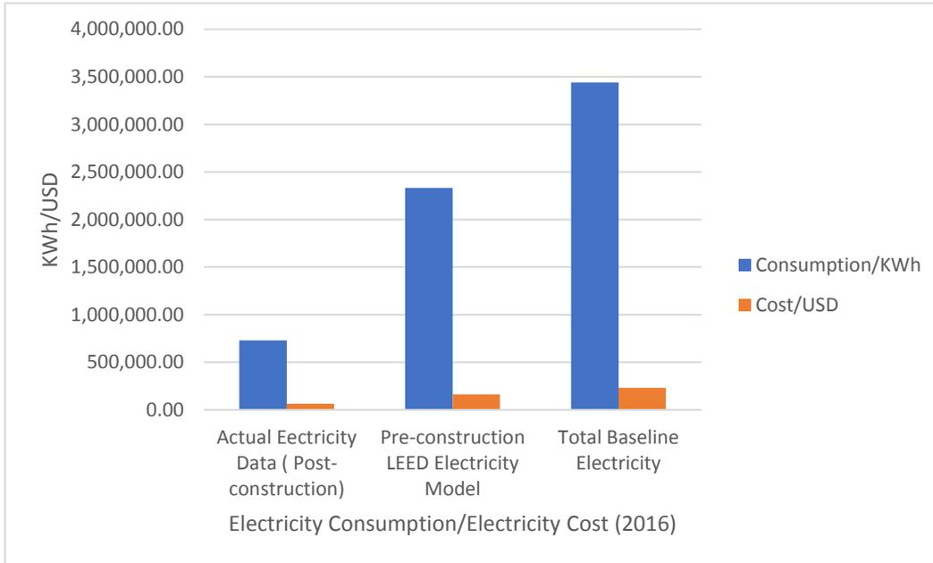
*Figure 5. Comparison Between Post-Occupancy Data and Pre-Construction LEED Model at Gary A. Ransdell Hall*
