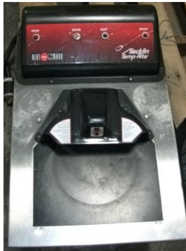
Figure 2. Original Inductive Heat Activator (Aladdin Temp-Rite, 2013)
