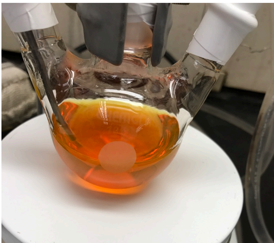
Figure 2.6. Image of completed nanorod reaction solution. It appears vivid orange with no precipitate particles floating in solution or settling at the bottom. This image also shows the 3-neck round bottom flask and how each joint is wrapped carefully with Teflon tape to ensure a moisture tight seal.
