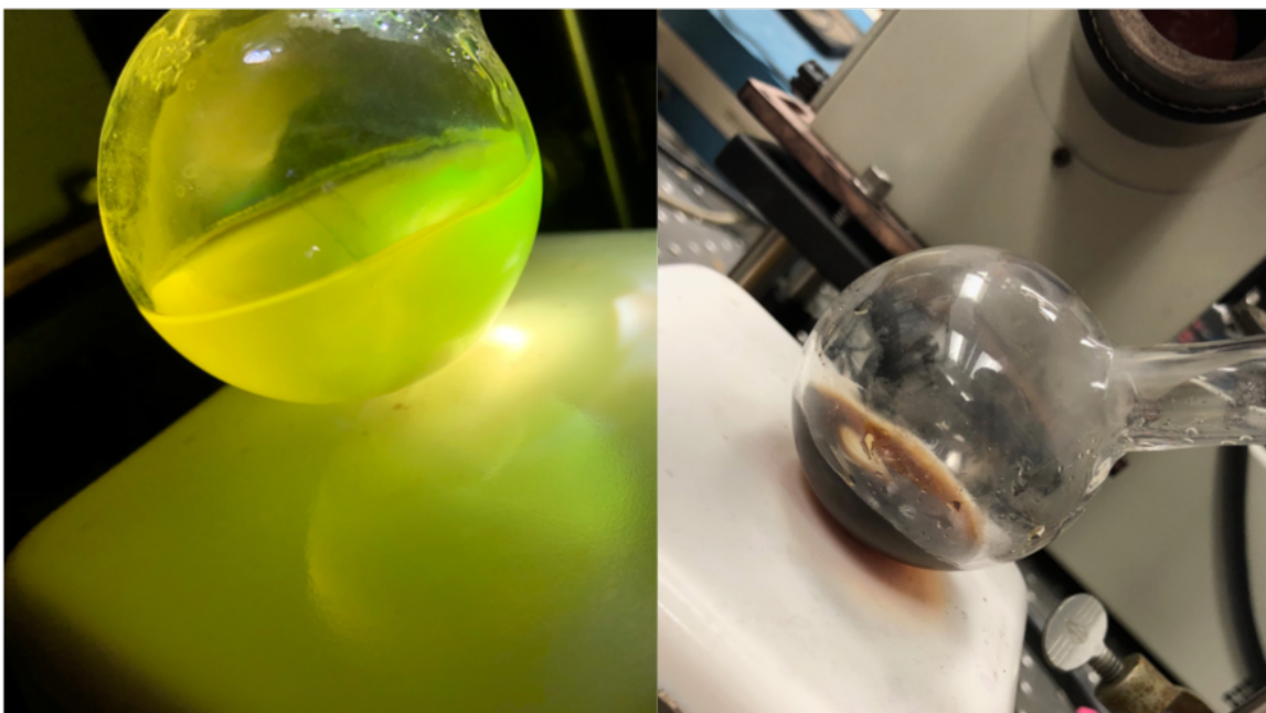
Figure 3.5. Image of the [BMIM]Tf 2 N solvent system photodeposition during (left) and after (right) the reaction.
