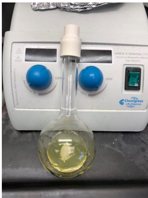
Figure 3.4. Image of the reaction vessel containing the [BMIM]Tf 2 N solvent system for the platinum photodeposition reaction.
