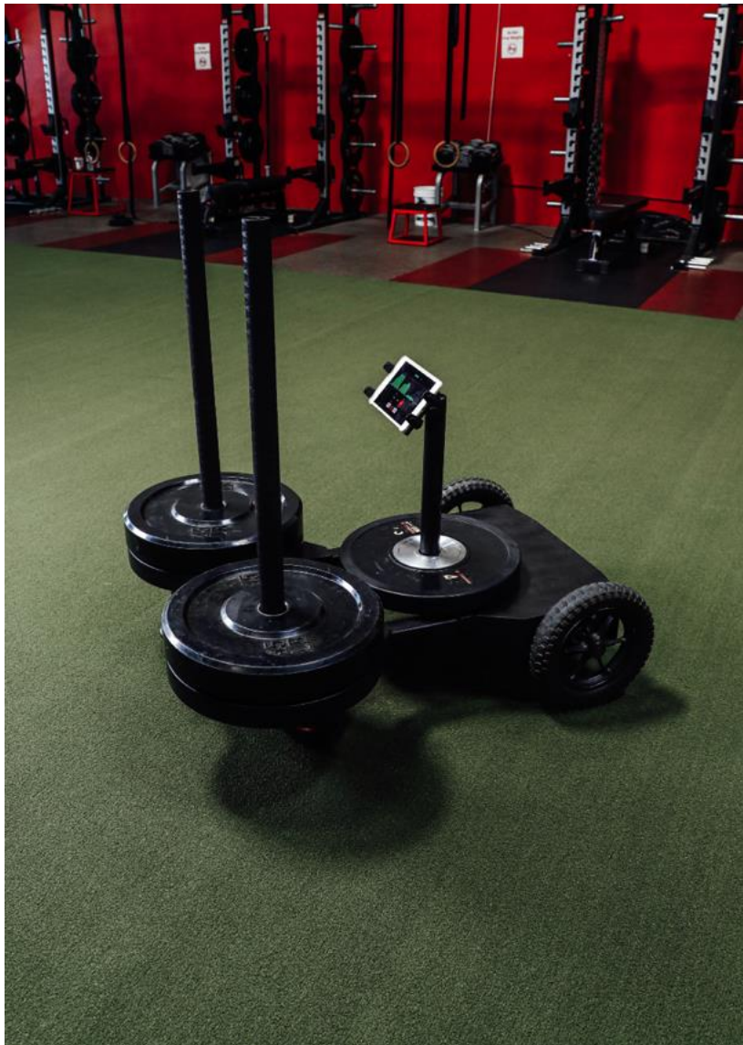
Figure 1. Smart Resisted-Sled, including RTF screen, loaded plate, and electromagnetic assembly.
