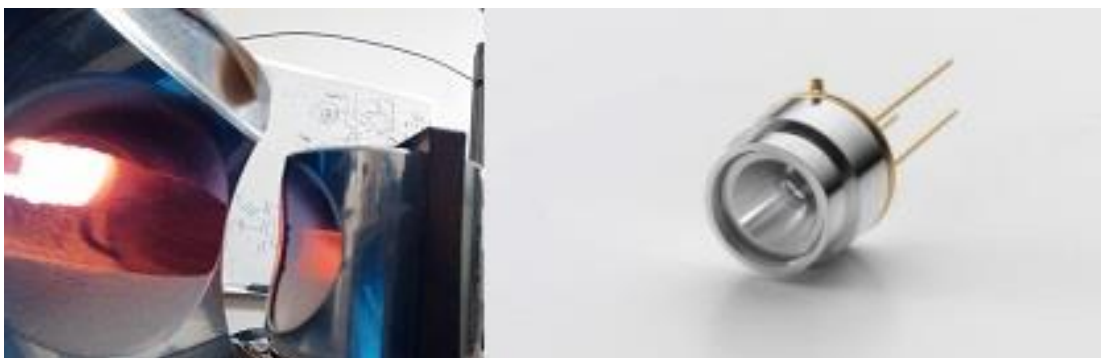
Figure 1. A heated coil IR source with a concave mirror (left), a micro-machined, electrically modulated thermal infrared emitter (right)
