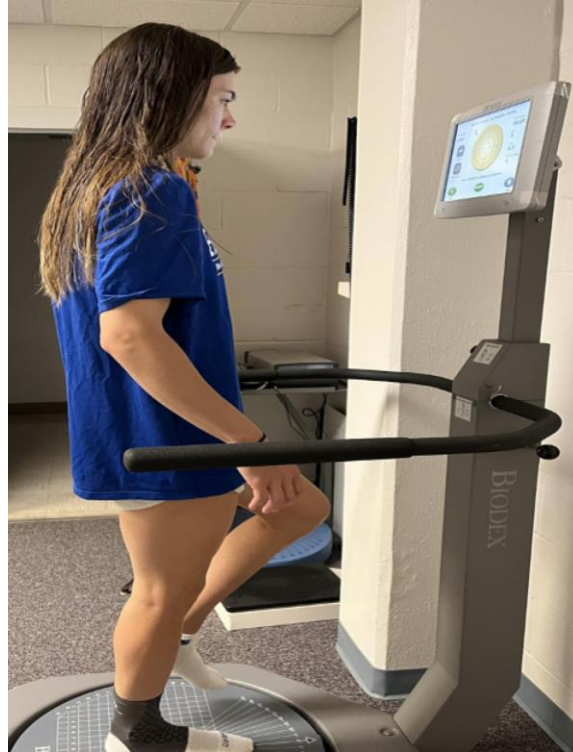
Figure 2. The Athletic Single Limb Stance Test on the Biodex Balance System. The participants were able to utilize visual feedback from the monitor in order to maintain their Center of Gravity on the platform.
