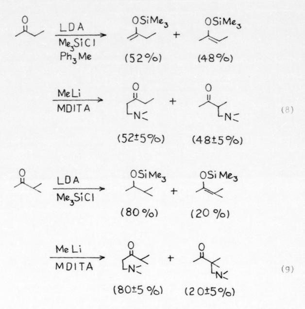
After treating the silyl ether with methyllithium, MDITA was added and the corresponding Mannich base was found regiospecifically. Observation of regiospecific behavior means that alkylation is faster than isomerization. This illustrated for 2-butanone (eqn. 10). Because of the overlap on the NMR spectra, the percentage of each isomer could not be
