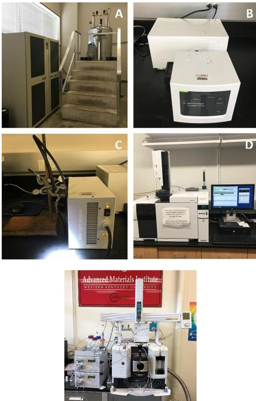
**Figure 2-1.** (A) JEOL ECA-500 MHz spectrometer. (B) Agilent 8454 diode array spectrometer. (C) SOLA SE II light engine, by Lumencor. (D) Agilent GC7820A/MS5977B. (E) Agilent 500 LCMS Ion Trap System.
