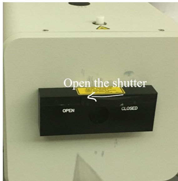
Figure B4. Opening the shutter on the front of the laser.
