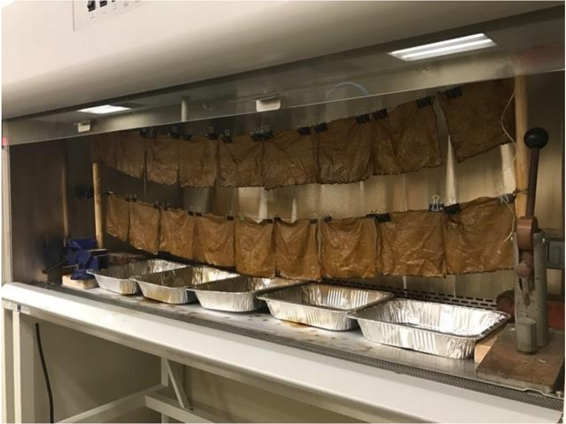
Figure A3.1. Laboratory experiment simulating a chili pepper fence used to deter elephants to detect capsaicinoid levels.
